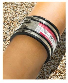
Peroxide-cured EPDM is recommended as continuous temperatures rise above 60°C for many years of leak-free service is assured up to temperatures of 125°C. Peroxide-cured EPMD has the same chemical compatibility as the standard VIPSeal range (sulphur-cured EPDM).
